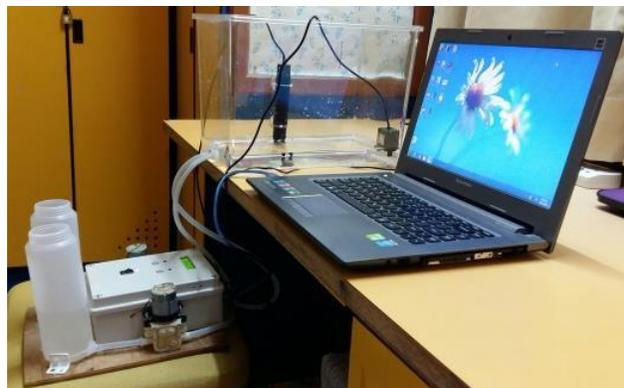
**Figure 6: Experiment Setup for Automated pH Regulator For Freshwater Prawn with pH Meter Pro**
