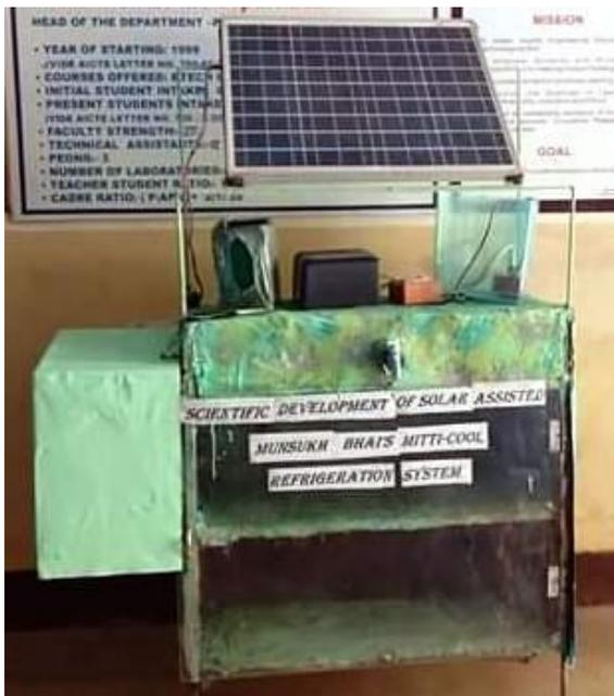
**Fig 5: Final prototype of Scientific Development of Mansukh Bhai's Mitti Cool Refrigeration System**
