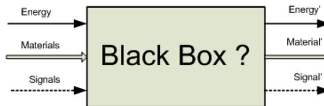
**Figure 2. Energy, material and signal conversion. Solution not yet known; tasks or functions that are explained based on input and output, Pahl and Beitz [10]**
